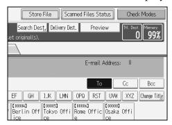
Up to 9 transmission or delivery results are displayed at the same time. Press [▲] or [▼] to switch between results.
